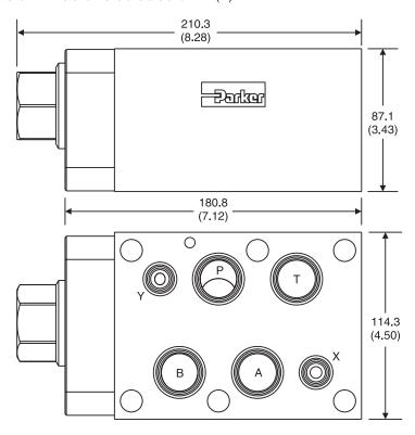
**CH08TT** — Inch equivalents for millimeter dimensions are shown in (\*\*)
