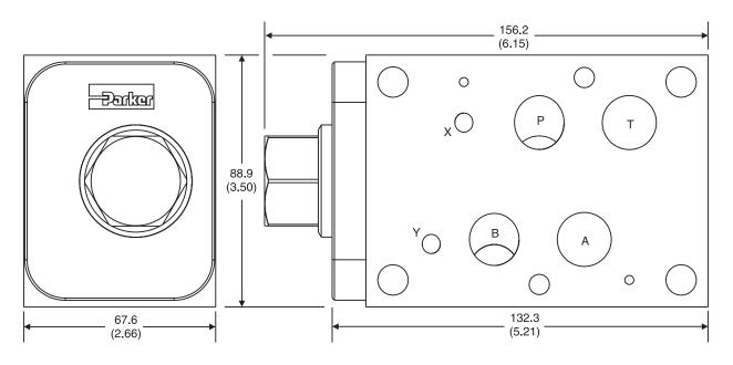
**CH07TT** — Inch equivalents for millimeter dimensions are shown in (\*\*)
